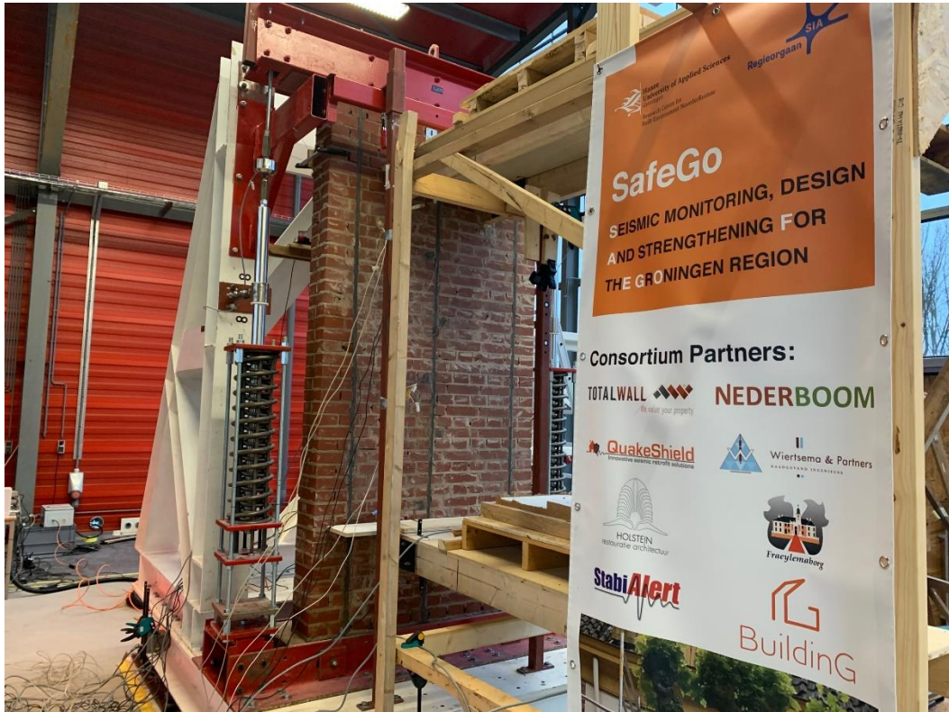
Figure 8. A solid masonry wall specimen being tested on the shake table (credit: SafeGO Project, NoorderRuimte).
