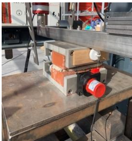
Figure 12. Brick stacks bond-wrench test example.
