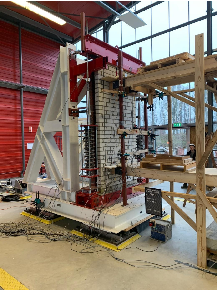
Figure 7. A cavity wall specimen being tested on the shake table.
