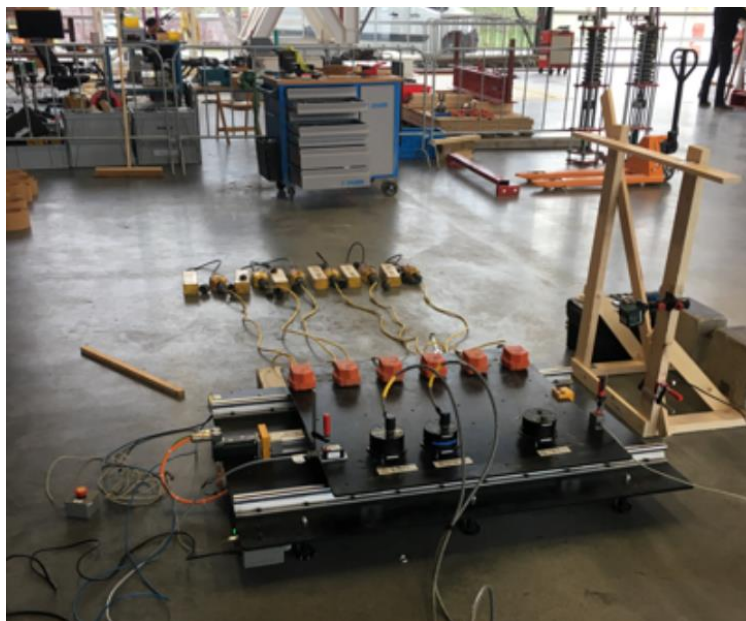
Figure 9. Small shake table used for testing KNMI accelerometers and geophones
