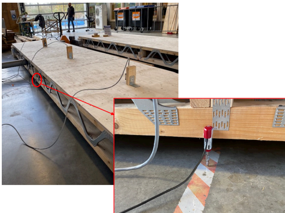
Figure 6. Displacement sensor (potentiometer) in the middle of the floor specimen
