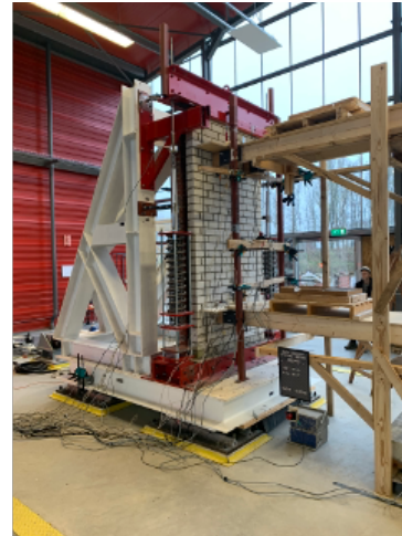
Figure 3. Shake table at BuildingG, dimensions (left) and picture from an actual testing on walls (right)
