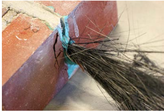
Figure 3.20: Post-experiment close-up of the loaded end of specimen PO-16-100-4 , showing the governing failure mechanism: CFRP rupture.
