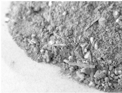
Figure 2.5: Dry polymer-modified mortar used for FRCM overlay.
