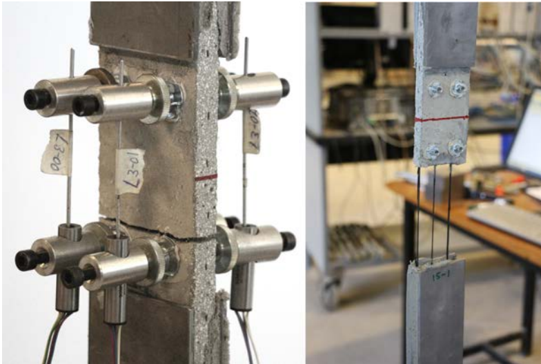
Figure 2.12: Damage on a FRCM coupon specimen during the tensile test: Crack formation (left) CFRP mesh slippage (right).
