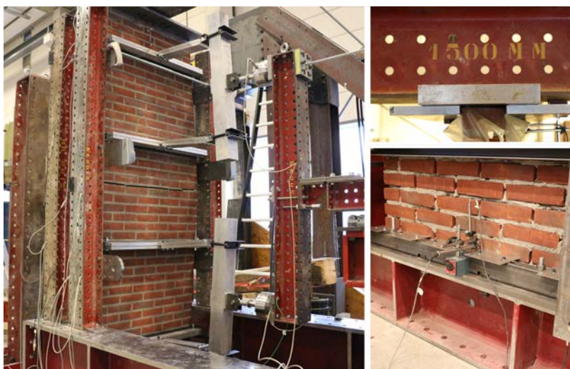
Figure 4.3: Detail photos of the setup: Loading beam for the 6-point bending configuration (left), top boundary condition of the wall (upper left), bottom boundary condition of the wall (bottom left).
