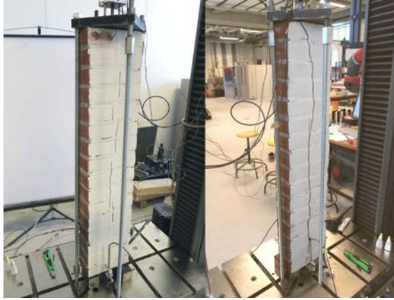
Figure 3.10: Marked hairline cracks of the front (left) and back side (right) of specimen Std-U-10, formed in the post-peak loading phase.
