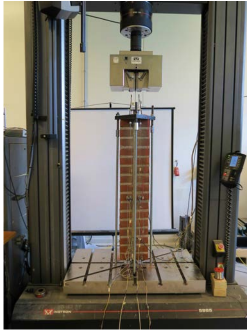
Figure 3.5: Test setup of the quasi-static DPT experimental campaign.
