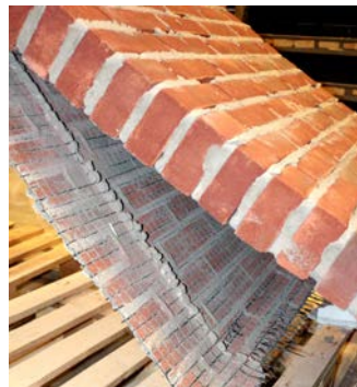
Figure 5.15: FRCM debonding failure of FRCM-1 .
