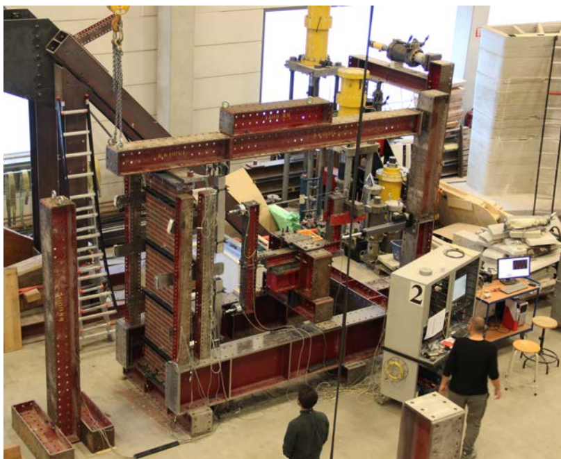
Figure 4.2: Test setup for the full-scale out-of-plane experimental campaign.
