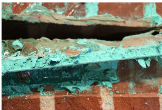
Figure 3.18: Close-up of specimen PO-12-100-2 after breaking the specimen apart post-experiment, showing the predominant cohesive failure.
